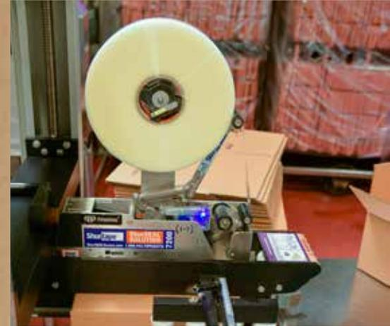
*The ShurSEAL Solution case sealing system was installed on lines in March 2014, and is used to seal the top and bottom flaps of nearly 90,000 corrugated cases per week.*
